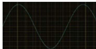
Filter On: Bandwidth = 5kHz (meets the 3kHz requirement of Energy Star)
