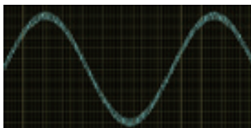
Filter Off : Bandwidth = 50kHz
