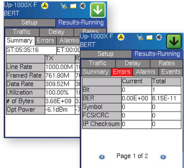
One traffic stream is transmitted across the network under test and bit-per-bit error checking is then performed on the received traffic. Service disruption measurements as well as CRC error checking are also performed. The BER test can be performed with a physical loop (or plug) at the far end (for a layer 1 circuit), or a second test unit or intelligent loopback device in Smart Loop or in Peer-to-Peer mode.
