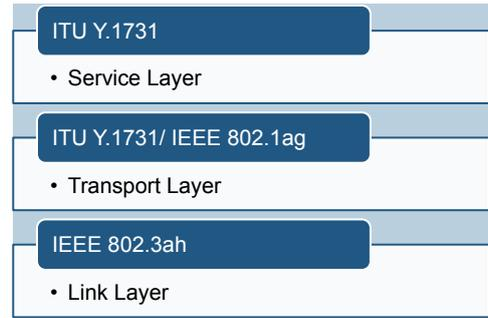
The TX130M+ offers a complete tool set for Link Level (IEEE 802.3ah) and Service Level (IEEE 802.1ag/ ITU- Y.1731) OAM for monitoring and maintaining carrier grade Ethernet services.
