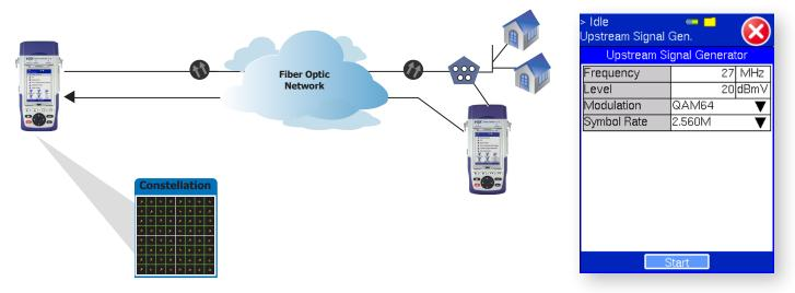
The CX150-D3+ transmits a reference signal of 5-65 MHz (Annex A) or 5-42 MHz (Annex B) to characterize the upstream. A choice of CW, QPSK, 16QAM, 64QAM and 256QAM modulation types with pre-defined symbol rates emulates DOCSIS cable modem transmission. Adjustable power level is useful to check amplifier performance resulting from overloading.
