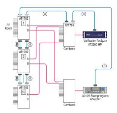
AT1600E/AT1700 series used with VeEX's Calan 3010H Sweep/Ingress system for remote return path ingress and sweep measurements.
