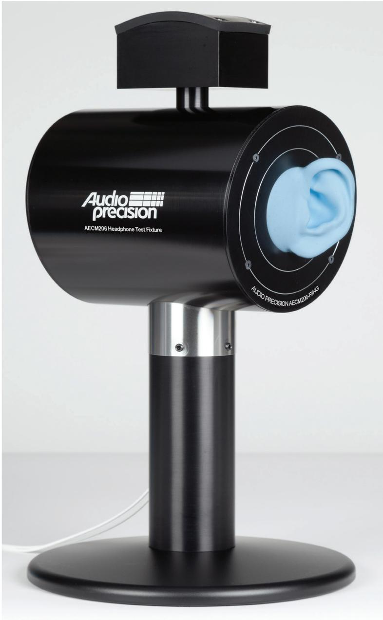
Headphone testing is complicated. The acoustic transmission paths involved in the close coupling of headphones, earphones and insert earphones (earbuds) to the ears must be considered; further, for measurements in noisy environments or testing ANC (active noise canceling) headphones, isolation is important.
