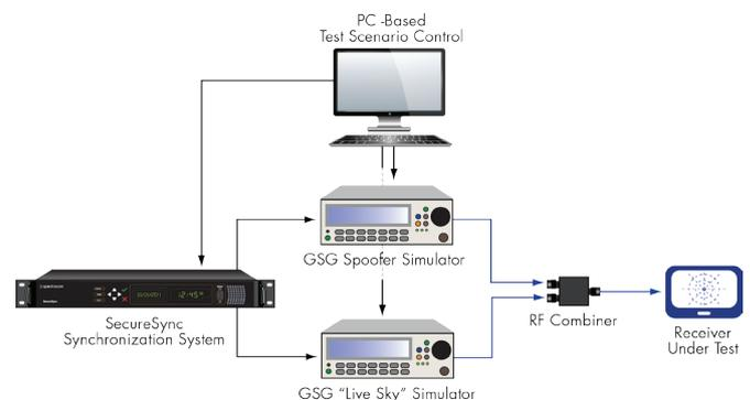
Spectracom's GNSS Vulnerability Test System consists of two simulators, a time and frequency synchronization unit, RF connectors, and PC control system. It comes with training and start-up assistance as well as a service plan so you get the most out of your testing program.
