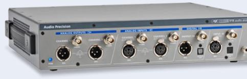
The APx515 is a fixed-configuration analyzer with a small footprint, designed for high-speed production, entry-level R&D and electro-acoustic applications.
